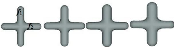
Figure 8. Level surfaces of a union of two cylinders by  $B_{U2}(f_1,f_2)=l$  with  $m_1=1$  and  $m_2=0.25$  for  $l=1, 1.2, 1.4$  and  $1.6$ ; On all of them,  $f_2$  dilates less than  $f_1$  because of  $m_2=0.25$ .
