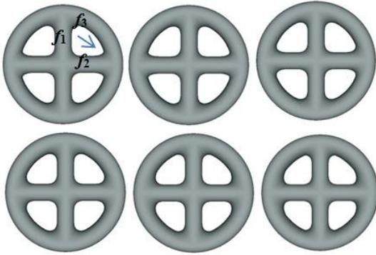
Figure 7. Sequential unions  $B_{A2}(B_{U2}(f_1,f_2), f_3)=1$  by (2) of  $B_{U2}(f_1,f_2)=1$ , intersecting cylinders, and  $f_3=1$ , a toroid. Varying  $m_2$  in  $B_{U2}(f_1, f_2)$  for  $f_2$  from 0.1, 0.5, 0.8, 1, 1.4 to 1.8 make the subsequent blends of  $f_2$  with  $f_3$  enlarging gradually without changing the shape of the transition on the intersecting region between cylinders as shown in surfaces from top left to bottom right.
