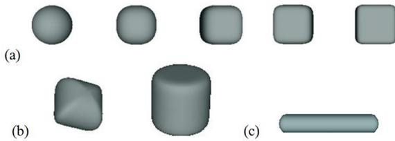
Figure 1. (a). Shapes of  $(|x/a|^n+|y/b|^n+|z/c|^n)^{1/n}=1$  where  $n$  varies from 2, 3, 5, 10, and 20. (b). Shapes of two super-quadrics. (c). Shape of a skeletal primitive (circular cylinder).
