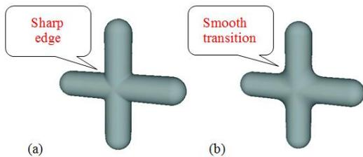
Figure 2. (a). A pure union  $Min$  of two cylinders, containing sharp edges. (b). A union blend of two cylinders, containing smooth transition generated automatically to remove sharp edges.
