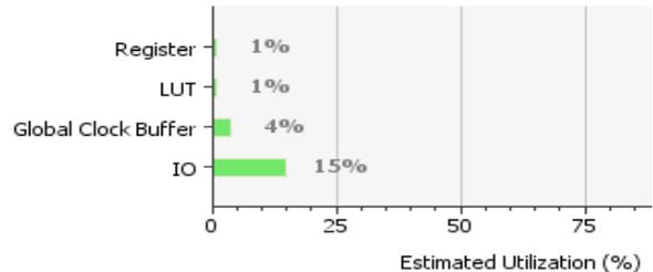
Figure 7. Low Power ALU Netlist Resource Usage Statistics
