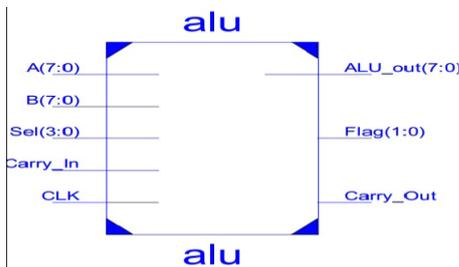
Figure. 3. Low Power ALU top level schematic
