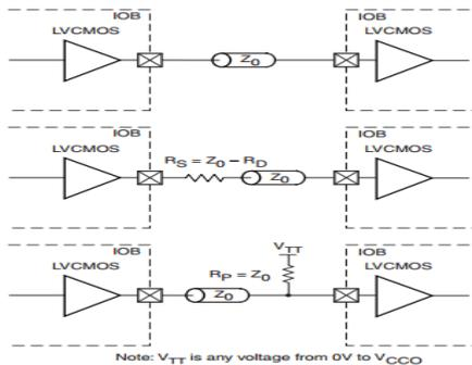
Figure 1. LVC MOS unidirectional termination [Source: Ref3]
